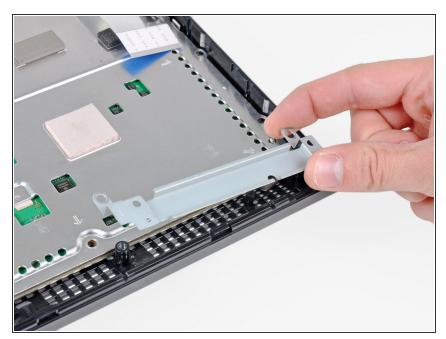
Remove the control board bracket.
