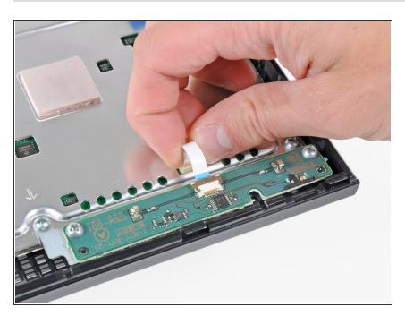
Pull the control board ribbon cable straight up and out of its socket on the motherboard.
