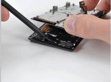
• Use the tip of a spudger to lift the speaker out of the screen housing.
