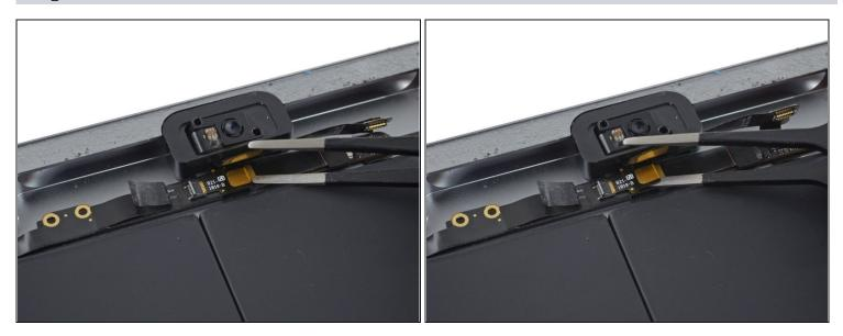
Slide the tip of a tweezer under the microphone cable to separate it from the adhesive holding it to the headphone jack cable.
