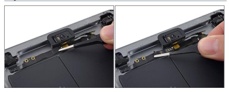
• Use a set of <u>tweezers</u> to peel up the small piece of tape covering the microphone cable connector.
