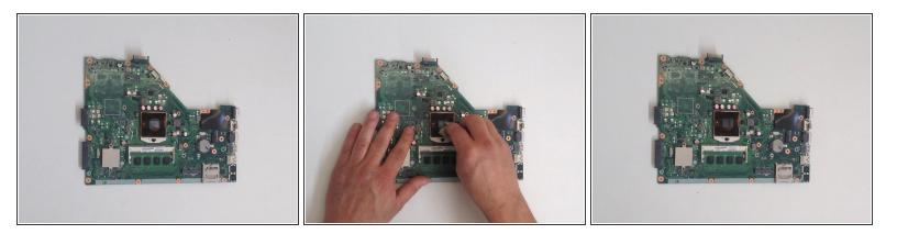
• Use the same technic to clean the surface of the processor from the old thermal compound
