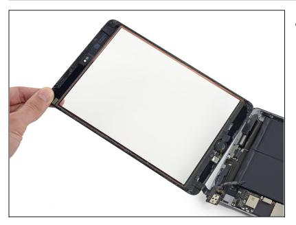
• Lift and remove the front panel assembly from the iPad.
