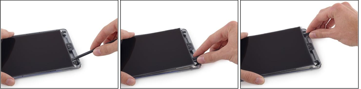
**i** The LCD is secured by mild adhesive that should be loosened before you flip the LCD up from its shield plate.
