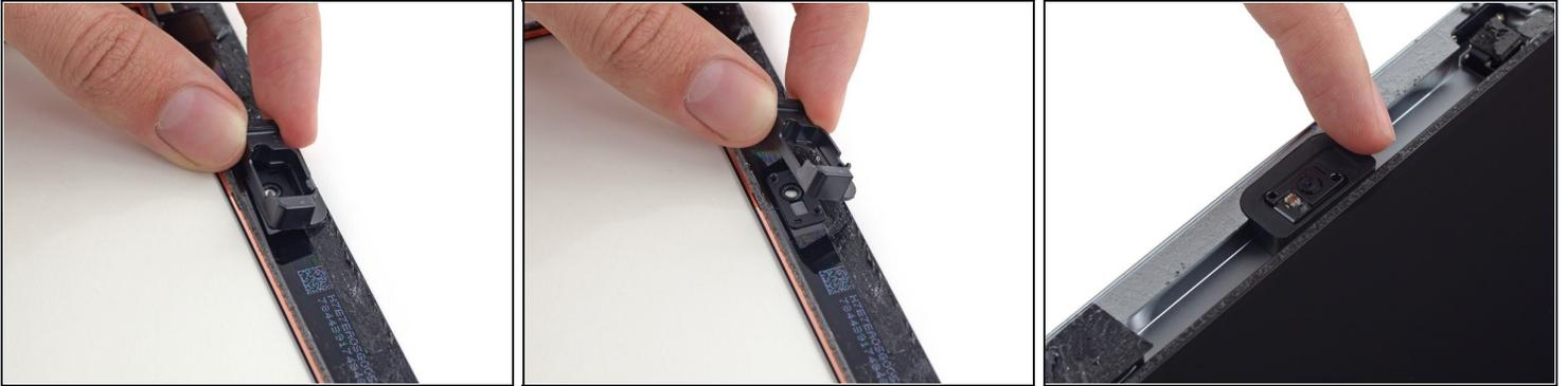
**i** The front-facing camera housing may stick to the front panel; peel up the housing and place it back over the camera to protect it.
