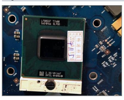
Insertion Force (ZIF) socket. If you (gently!) try to pull the CPU out of its socket, you will find that it does not budge. You first need to release the chip from the socket. Turn the screw on the CPU socket 180 degrees counter-clockwise to release the old CPU. Then pull up on the CPU chip to remove it.
