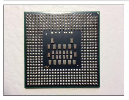
Insert your new CPU into the ZIF socket. Note that two pins are missing from one corner of the grid. Match that corner with the corner of the socket that is missing the corresponding holes. Drop the chip in; it should go in without effort. Rotate the screw on the socket 180 degrees clockwise to lock the new CPU in place.
