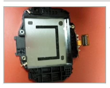
Using a small pliers and a small flat screwdriver the battery housing comes out easily.
