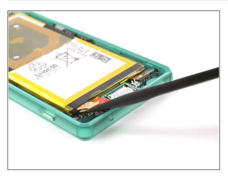
Disconnect the battery flex cable.
