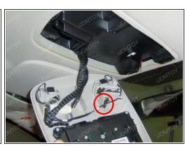
• Wire up the LED lights in parallel. Use some electrical tape to secure the connections. Route the wires through the front map light assembly to complete the wiring portion.
