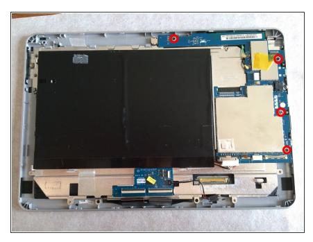
• Remove the four Phillips screws securing the motherboard.
