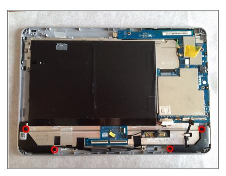
Remove the four Phillips screws securing the two speakers.
