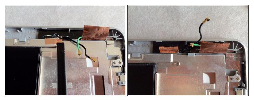
• Peel off coper tapes from the metal plate.
