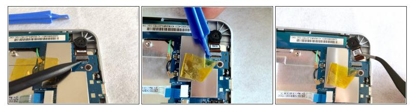
• Pry up the black bar to unlock the camera connector
