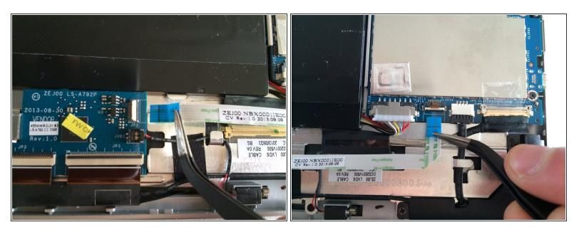
• Remove the flex cable pulling it out its two connectors.
