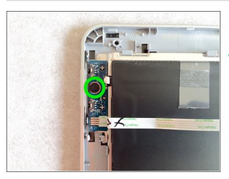
Remove the single Phillips 000 screw securing the volume buttons circuit board.
