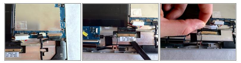
• Peel off the cristal tape pieces upon each connector side.
