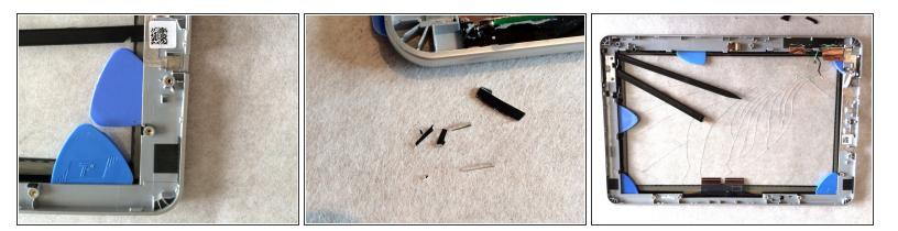
• Introduce plastic opening tools, turning around to separate frame and touchscreen.
