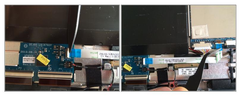
• Pry up the white bars to unlock the two connectors.
