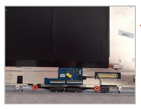
Remove two remaining Phillips screws securing the metal plate.
