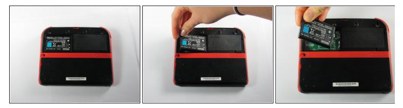
• Remove the battery from its housing by lifting it up from the side closest to the outside edge.
