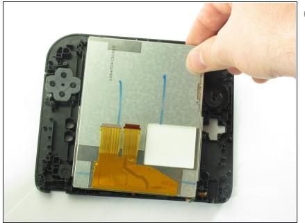
(i) Ensure that the ribbon cables connecting the screen to the motherboard have been disconnected before removing the screen from the front panel casing.
