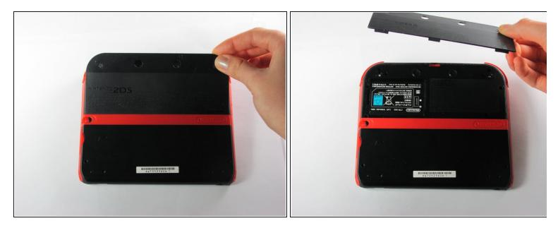
• Hinge the upper rear panel upwards and outwards to remove it.
