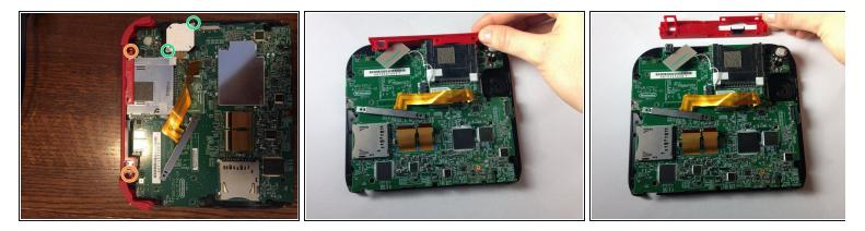
*i* The top panel can only be removed when the mother board is not secured.
