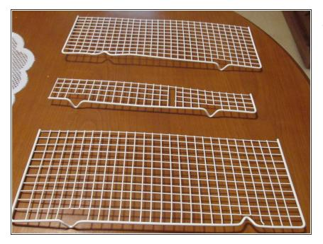
measure first and choose racks that over fit half the drawer space. Now its important before cutting you decide the TOP. You must place the racks so as to make the left to right cross wires sit ON TOP of the long run wires. This helps glasses not to slide down to the front. Angle grind the surplus edge off each rack. Keep one for middle rack.
