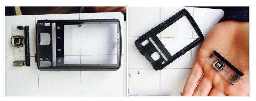
Remove buttons from back case of screen cover. Replace with new set of buttons.
