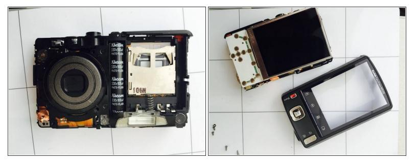
• This is what the camera should look like with all screws are removed. Flip camera over to carefully remove the screen cover.
