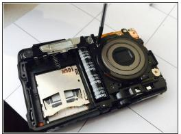
To get to control buttons, use a Phillips Head screw driver to unscrew the three screws near lens.
