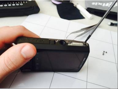
Use a Philips Head screw driver to unscrew the sides of the camera. There are two screws on each side except for the top of the camera. Carefully remove face plate of camera. Place alongside near screws.
