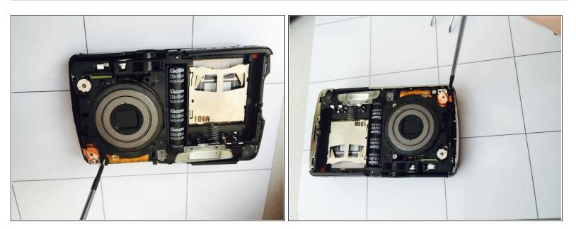
Remove additional screws near lens.
