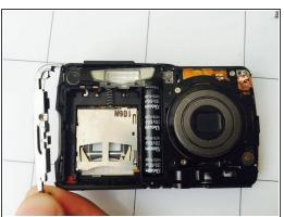
Unscrew the screw near the rechargeable battery compartment. The metal piece then can be removed.
