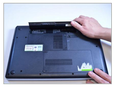
Carefully remove the battery from its compartment.
