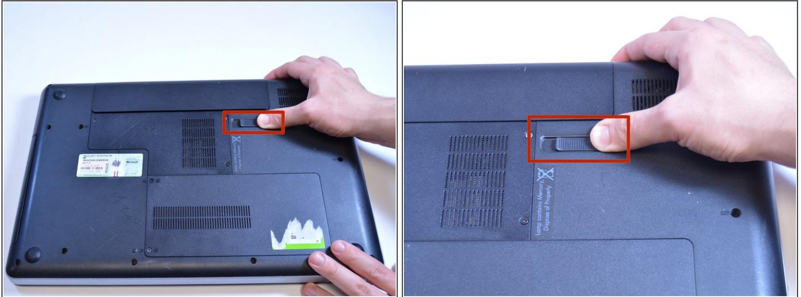
**⚠** Removing the battery while the laptop is still on may corrupt your files.
