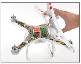
• Lift up on the top portion of the shell and set it on its side.
