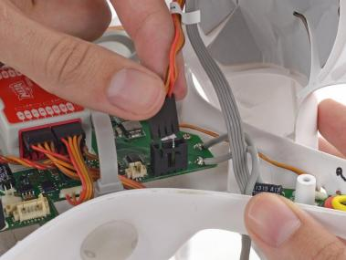
Lift the GPS cable molex connector up out of its socket on the main board.
