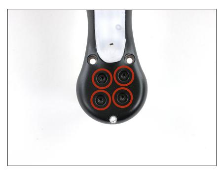
Remove the four 2mm hex motor bolts.
