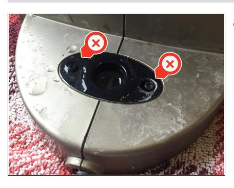
Remove the two TR10 screws from the bottom part
