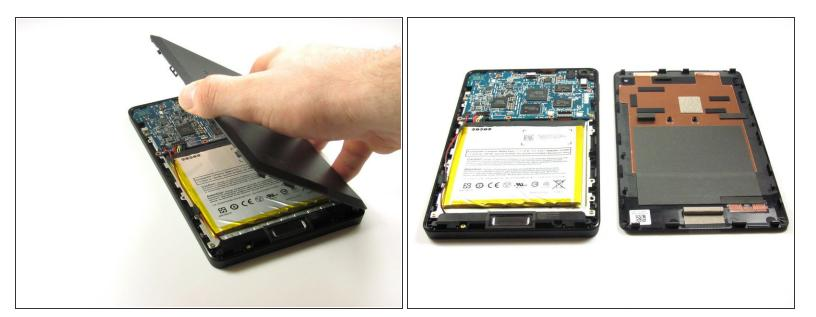
• Carefully separate the back panel from the rest of the device internals.
