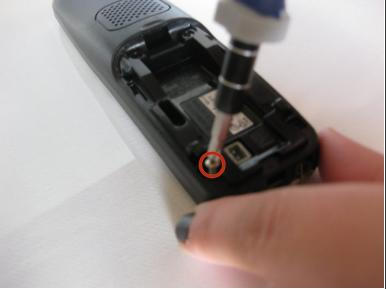
Using a Phillips #1 screwdriver, remove the two .9 mm screws on the back of the device on each side of the battery pack.
