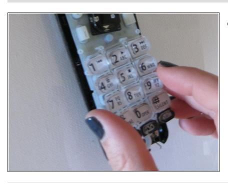
Gently remove the loose keyboard from the lined gel casing located under the front housing of the front of the phone.
