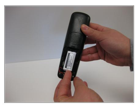
Remove the white battery pack from the battery compartment.
