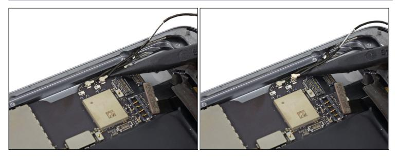
• Use the point of a spudger to lift the left antenna cable connector straight up off of its socket on the logic board.
