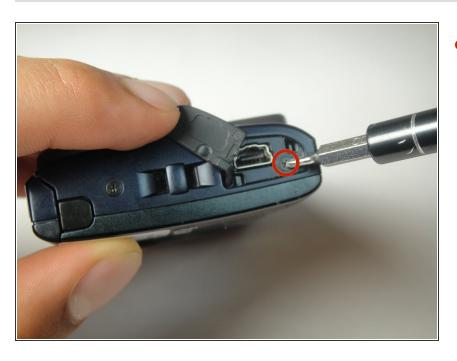
Remove the 5.00 mm screw from behind the cover.
