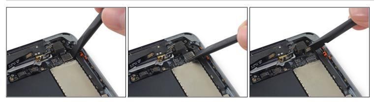
• Use the flat end of a spudger to disconnect the rear-facing camera cable from its socket on the logic board.
