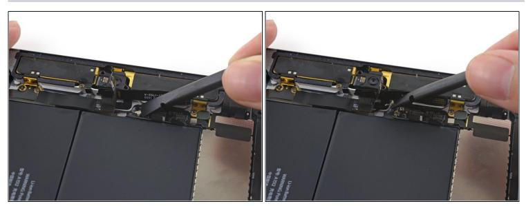
• Use the flat end of a spudger to lift the top left antenna cable connector up from its socket on the logic board.
