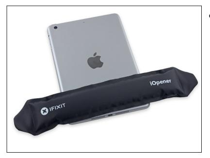
• Place a heated iOpener on the bottom of the rear case for one minute.
