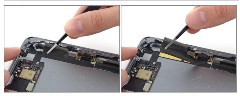
• Peel up the tape covering the Lightning connector cable.
