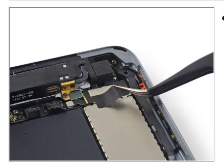
• Remove any tape from the rear-facing camera cable bracket.
