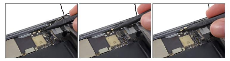
• Use the point of a spudger to lift the two antenna cable connectors straight up off of their sockets on the logic board.
