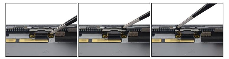
• Use a set of tweezers to remove the small plastic covers on the screws in the Lightning connector housing.
