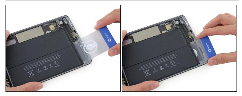
• Remove the plastic card and insert it under the cell nearest the edge of the case.
