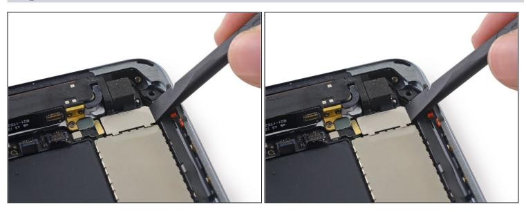
• Use a plastic opening tool to push the rear-facing camera cable bracket to the left.
