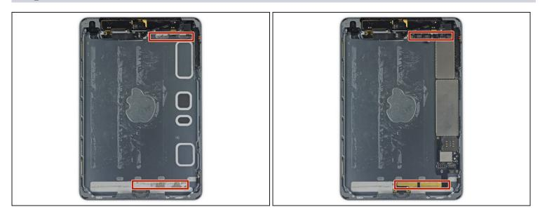
i The logic board is held in place by two strips of adhesive.
