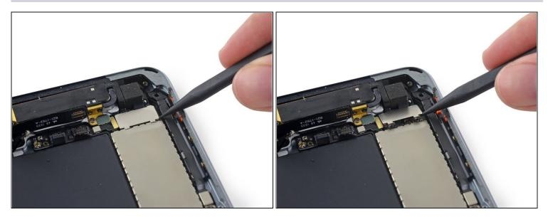
• Use the tip of a spudger to lift the front edge of the bracket.
