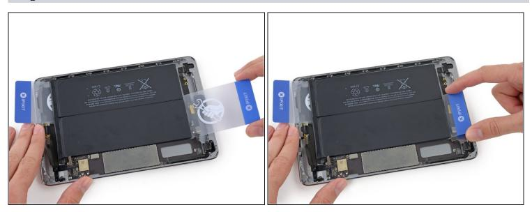
• Insert a second plastic card beneath the battery on the logic board side near the frontfacing camera.
