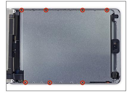
• Remove the seven 1.8 mm Phillips #00 screws from the LCD shield plate.
