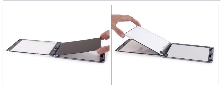
🗥 Do not attempt to fully remove the LCD. It is still connected to the iPad by several cables at the home button end. Lift only from the front-facing camera end.
