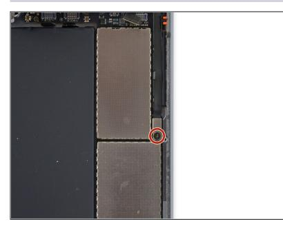
• Remove the 1.8 mm Phillips #00 screw securing the case button cable bracket.
