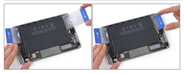
• Remove the second card and reinsert it under the battery near the headphone jack.
