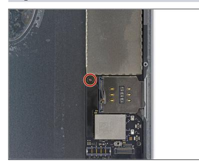
• Remove the single 1.3 mm Phillips #00 screw from the logic board.
