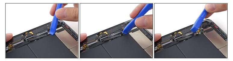
• Use a plastic opening tool to fold the front-facing camera cable clips outward, away from the cable, to free the cable connector.
