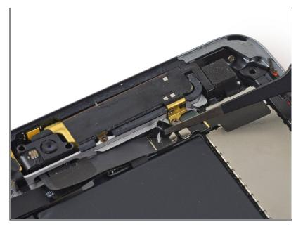
• Use a set of tweezers to remove any tape covering the frontfacing camera cable clips.
