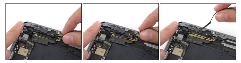
• Lift the antenna cable tape up from behind the right speaker.
