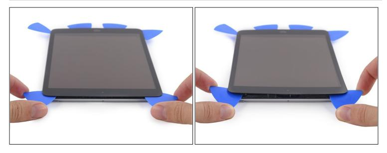
A Be very careful with this step. Take your time and ensure the adhesive is hot and soft, and that you've been through all of the adhesive with an opening pick. Don't be afraid to stop and reheat.
