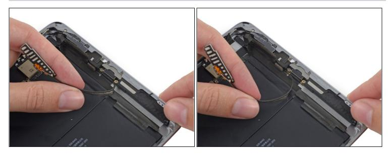
• Pull the antenna cable from the clip behind the Lightning connector.
