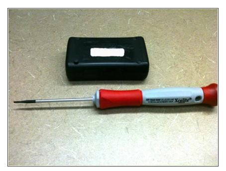
Use a small tip flat blade screw driver to remove the rubber plugs.
