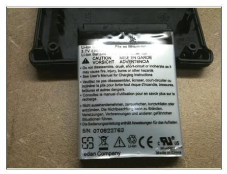
Old battery. No numbers just 3.7 volt 890mAh. Very difficult to figure out. I found a Sony Erricson J100, J220, W710, W810, Z300, Z710 battery that fits perfectly.
