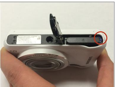
Open the camera battery terminal that can be found on lower right corner of the camera.
