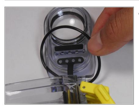
Now that the O-ring is out of the groove, remove the O-ring from the lid.
