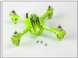
Use a Phillips #000 screwdriver to remove the three screws securing the lower body to the frame.
