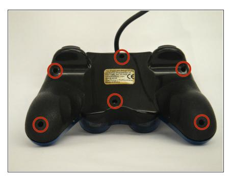
Remove the six 7 mm Phillips screws from the rear cover.
