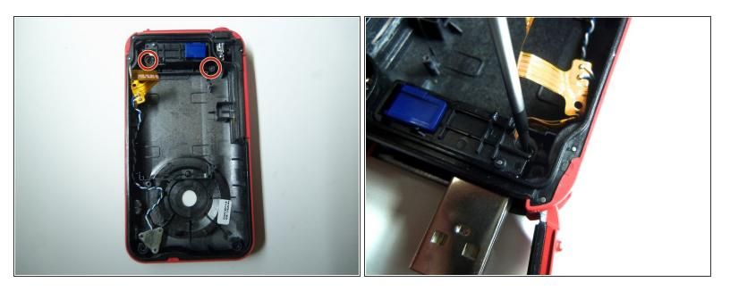
• Remove both screws from the USB port using a Phillips #00 screwdriver.
