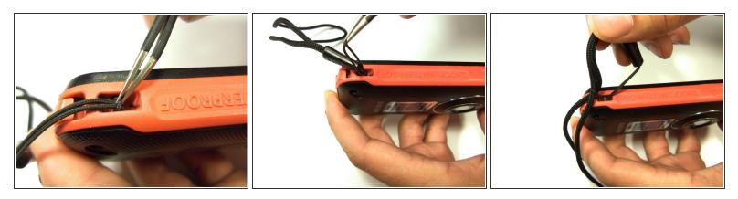
• To remove the wristband of the device, grab the middle loop and pull the band through.
