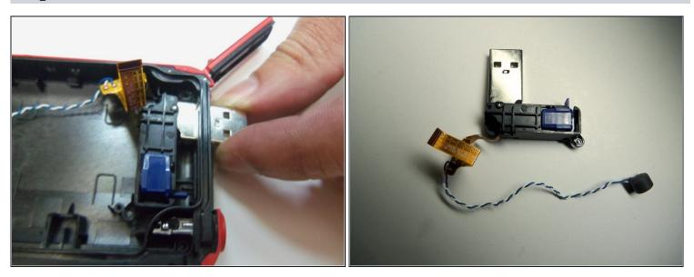
• Push the USB port inside the case to remove it from the device.
