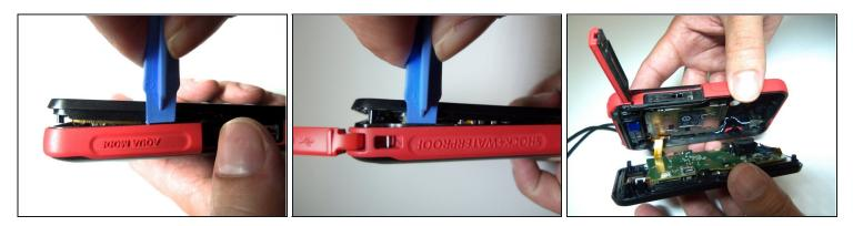
• Use the iFixit opening tool on both sides on the device. Pry apart both sections with light force.
