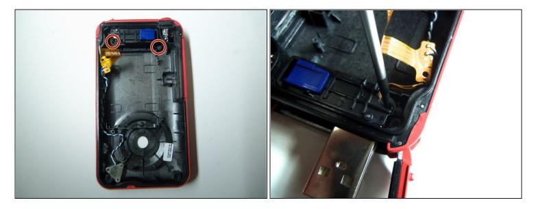
• Remove both screws from the USB port using a Phillips #00 screwdriver.
