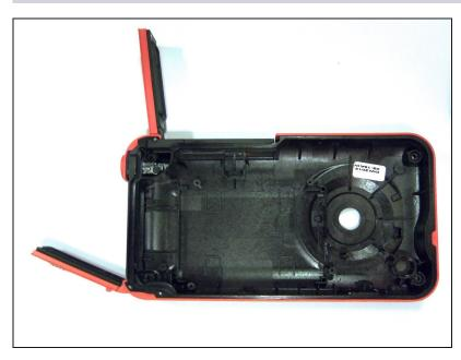
• The front case is separated from the rest of the device.
