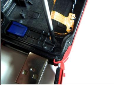
Remove both screws from the USB port using a Phillips #00 screwdriver.
