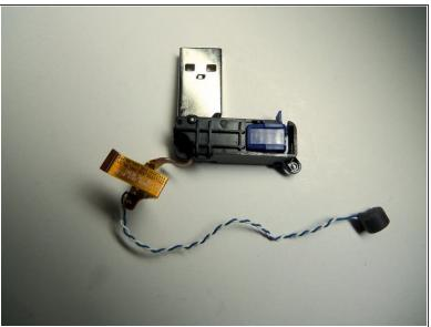
Push the USB port inside the case to remove it from the device.
