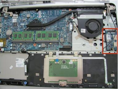
Pull back the tape that is securing the cable to the USB board.
