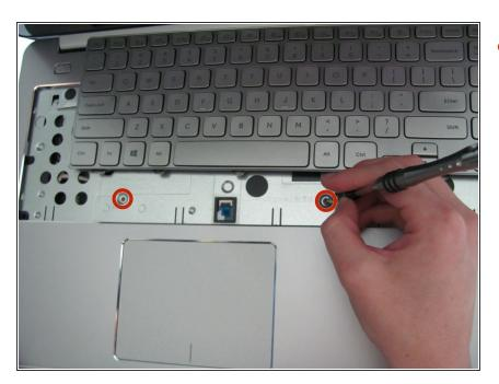
Unscrew the two black 5 mm screws underneath the keyboard using a Phillips head screwdriver.
