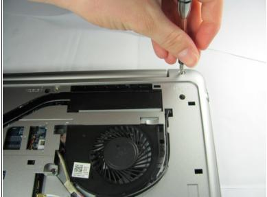
Flip the computer and remove the two silver 5 mm screws on the corners of the base cover with the Phillips head screwdriver.
