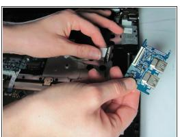
• Lift the black latch and remove the USB cable from the USB board.
