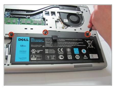
Remove the three 5mm Phillips #0 screws that keep the battery connected to the computer.
