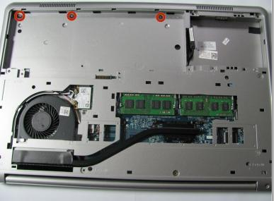
Remove the three silver 2 mm screws (with large flat circular heads) from where the battery was taken out with the Phillips head screwdriver.
