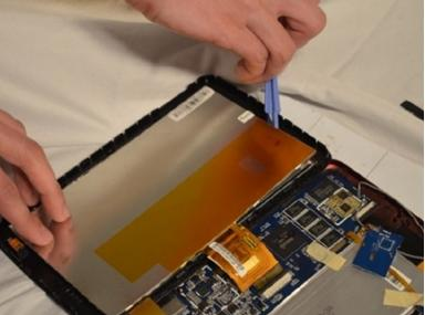
Insert the plastic opening tool into the wedge and pry it open.
