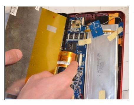
Open the latch and pull to remove the LCD.
