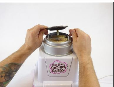
• Firmly grip the extractor head and slowly lift vertically to remove from the device.
