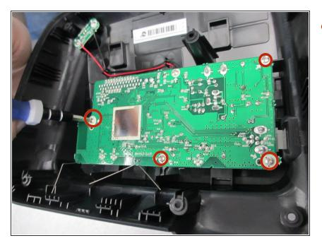
Unscrew bottom shell circuit board screws (Head size: 4mm Length: 8.6mm).
