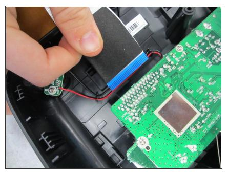
• Disconnect the ribbon cable from the bottom shell circuit board.
