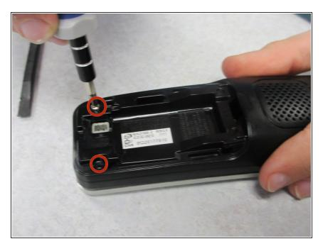
Remove the battery, and unscrew the two screws (Head Size: 4mm Length: 8.6 mm).
