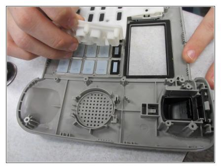
• Remove rubber keyboard underlay from top shell.
