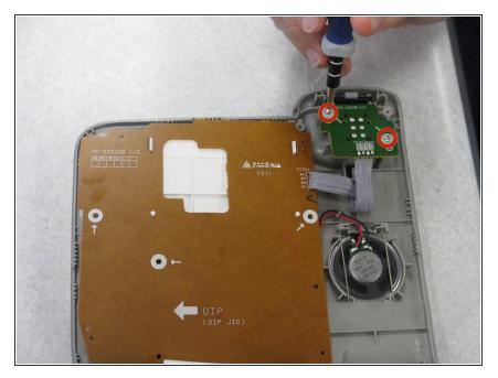
Unscrew the 2 screws (Head Size: 4mm Length: 8.66) on the small circuit board in the top shell.
