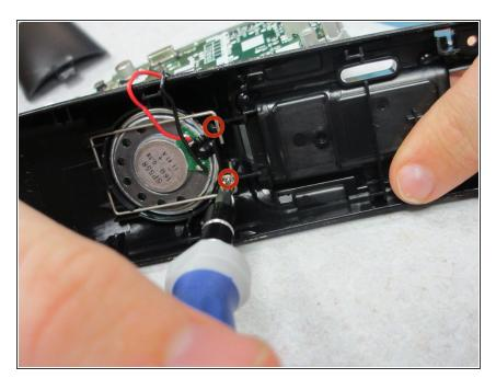
Unscrew the two screws (Head Size: 4mm Length: 8.6mm) on the bottom shell keeping the speaker locking pin in place.
