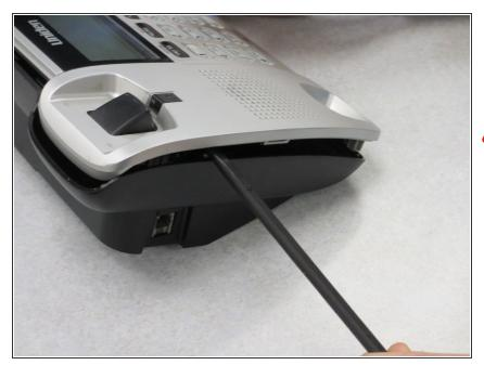
Using the spudger, separate the top shell of the base from the bottom shell from the base.
