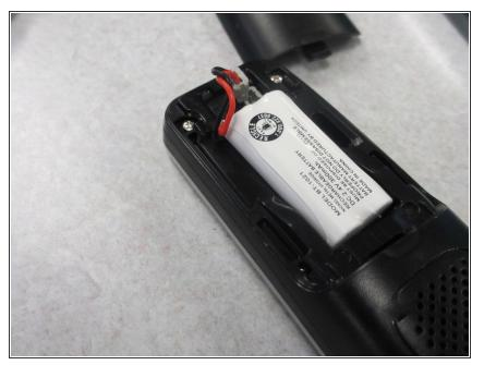
• Slide the battery cover off of the handset, and unplug the battery.
