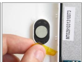
Remove the tape holding the speaker in its socket.
