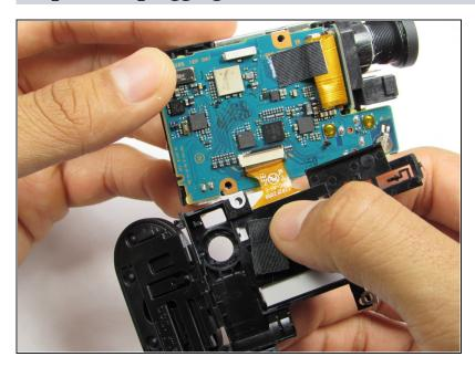
A ribbon cable attaches the LCD to the circuit board, this can be removed by gently pulling on the cable as close to the end that attaches to the circuit board as possible.
