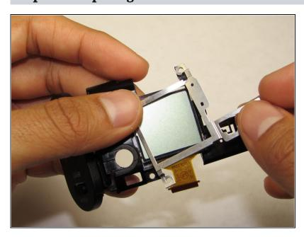
Gently remove the metal piece by pulling out to the right on the upper right corner first, and then on the bottom left corner.
