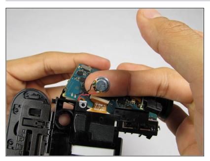
Pry the speaker out from its slot gently, careful not to rip the wires from the circuit board.
