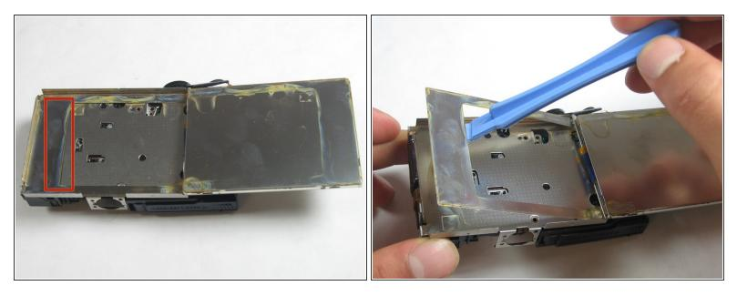
• Remove the metal plate with the plastic opening tool.
