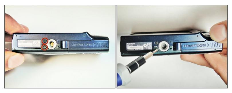
Remove the two 5.00 mm screws in the bottom of the casing with a Philips #000 screwdriver
