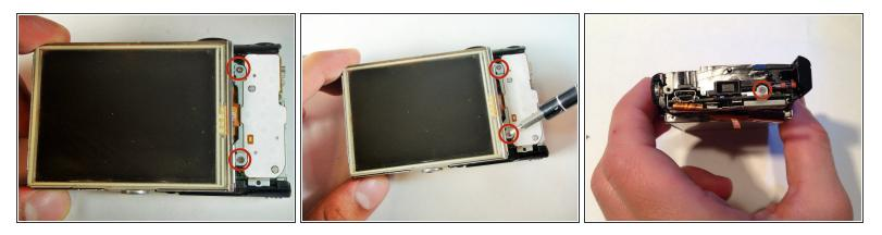
Remove the three 5 mm screws
