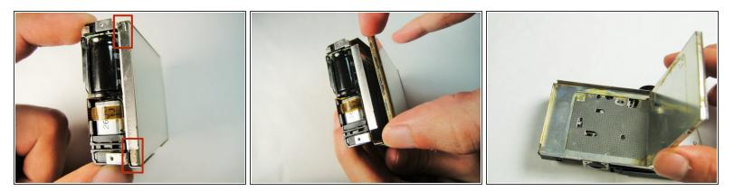
• Remove the screen by pulling at the two points as shown.
