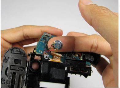
Remove the tape holding the speaker down.
