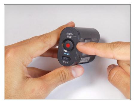
To access the battery, gently pry open the rear cover of the action cam.
