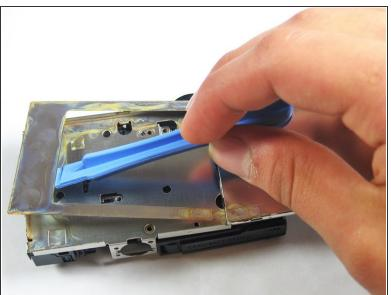
Lift the metal plate with the plastic opening tool.
