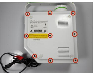
Flip the projector onto its back and unscrew the nine 15mm screws using the Phillips #0 screw driver.
