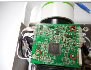
Unscrew the three 6 mm screws from the motherboard with the Phillips #0 screwdriver.
