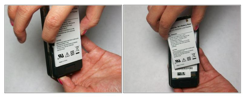
• Pinch the battery from both sides and lift the battery to remove it.
