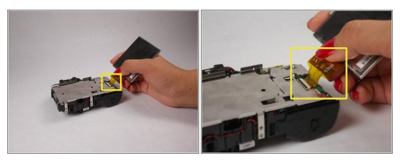
While the LCD screen is loose and unattached, there is a latch that is holding the ribbon in place.
