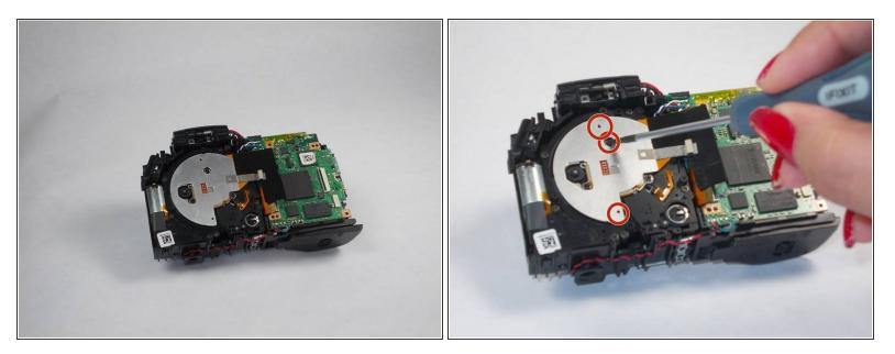
• Remove the 3 (3.10 mm) screws that are located on the back of the lens cover.
