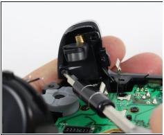
• Unscrew the two 7mm T6 Hex screws located on underside the triggers.
