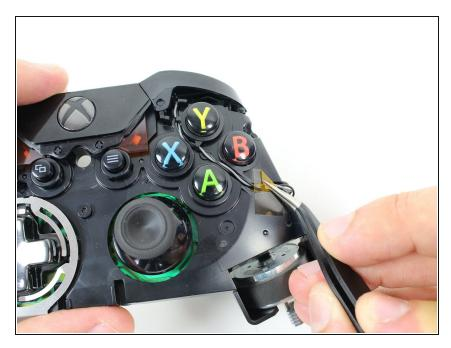
Remove the yellow tape holding the wires in place on the front of the controller.
