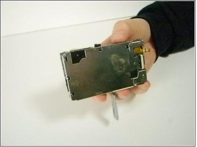
Slide the right side of the LCD screen clockwise, which will push it off the camera. The rest of the screen should come off with it with ease. To reassemble your device, follow these instructions in reverse order.
