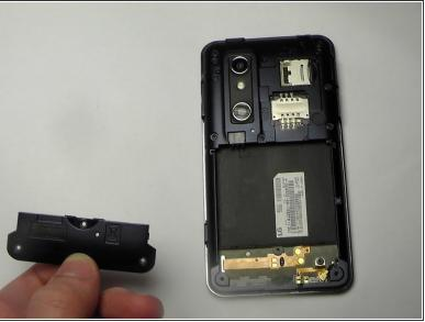
Use your finger or opening tool to wedge the speaker out starting at the small notch at the bottom of the phone.
