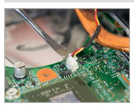
Use your fingers or a spudger to remove the power pin connecting the fan to the laptop by pulling it straight up off the motherboard.
