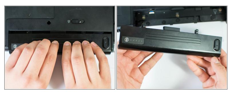
Remove the battery using two hands and pull it away from the computer.
