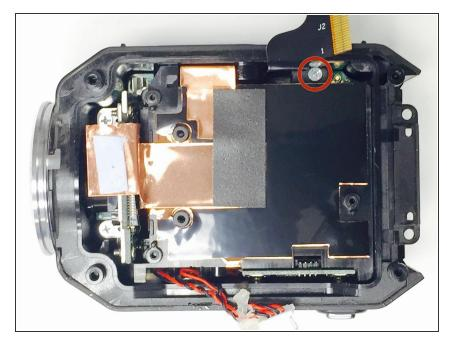
Once the circuit board is removed, you will want to remove the Phillips screw (3mm headsize x 2 mm length) near the ribbon cable. ONLY REMOVE THIS ONE SCREW.
