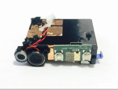
Now you should be able to gently remove the battery housing out of the device. If you are having difficulty getting the battery housing to come out, you may want to use the plastic opening tool to help get it started.
