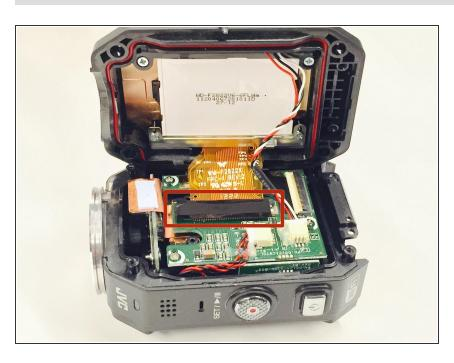
Carefully lift open the camera from the side of the device with the record and play buttons. Then remove the black cover tape by gently peeling it off. Make sure to save this tape as you may need it when you re-assemble the device.
