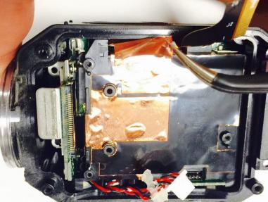
Carefully remove both the top and bottom copper strips by gently pulling them off with the tweezers.
