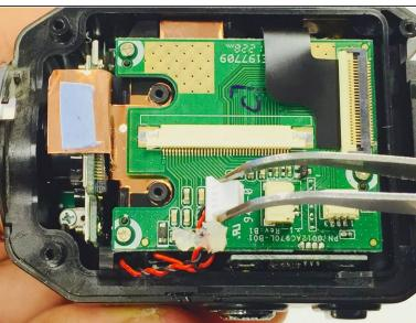
Carefully peel off the glue holding the red and black braided wire down to the circuit board. Then
