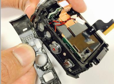
Use the plastic opening tool to gently remove the top cover from the camera. It is glued on, so you
