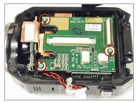
Remove the three Phillips screws (3mm headsize x 2mm length) from the circuit board. After you remove the screws, you can then remove the green circuit board by lifting it up out of the device case. You may want to use the plastic opening tool to get start lifting the circuit board.
